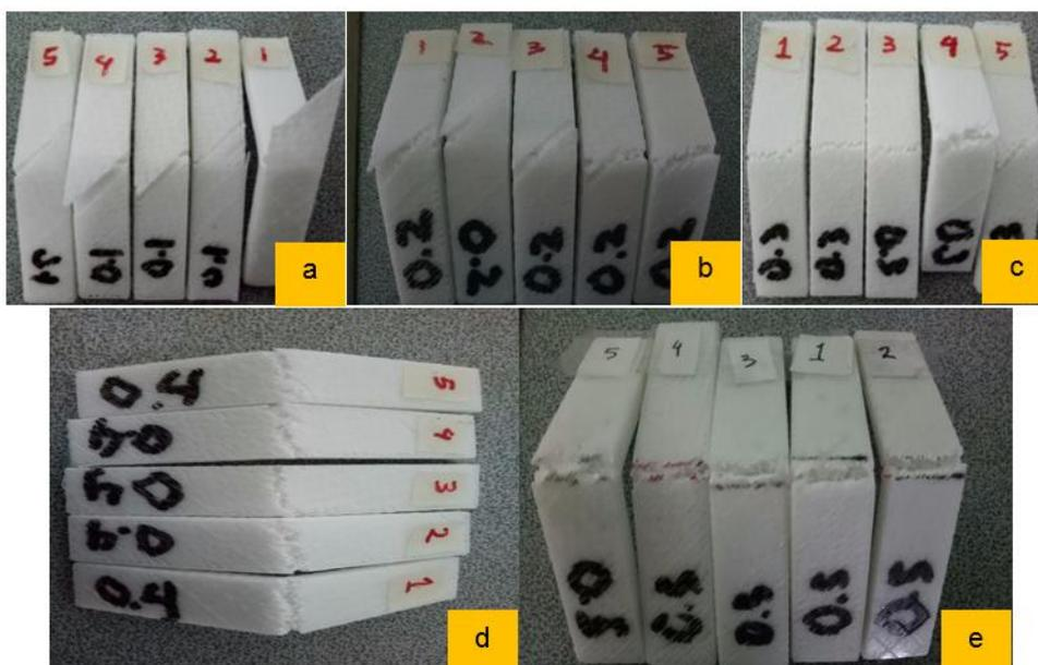
**Figure 10.** Fracture characteristics of PLA samples with different layer thickness: (a) 0.1mm, (b) 0.2mm, (c) 0.3mm, (d) 0.4mm, (e) 0.5mm.
