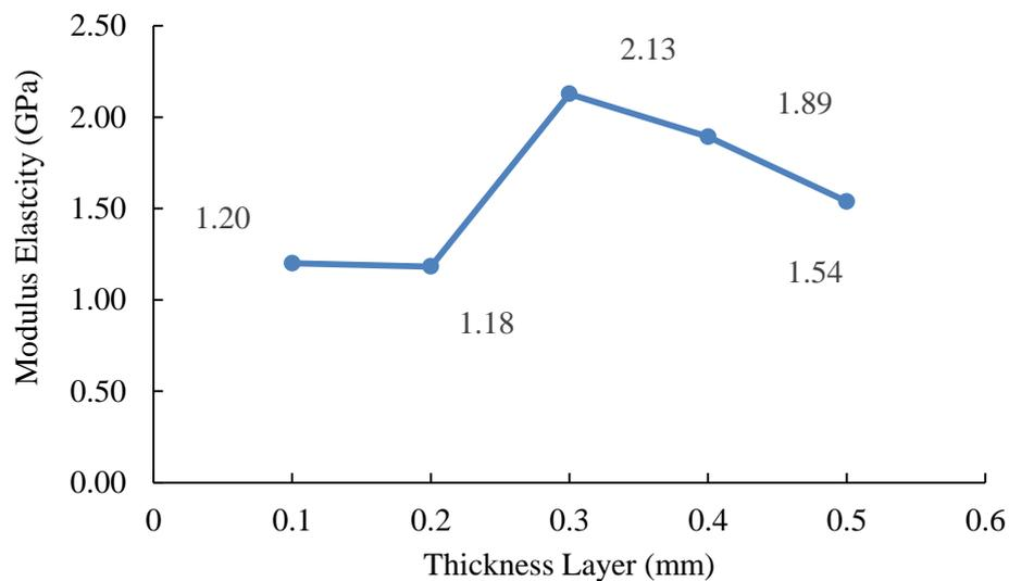
**Figure 8.** Graphical comparison of average maximum flexural stiffness ( $E_f$ ) for the flexurel specimens as a function of layer thickness.
