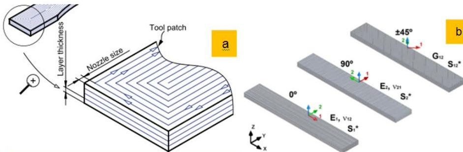
**Figure 5.** (a) Layer thickness and perimeter raster [17], (b) illustration of printing orientations [18].
