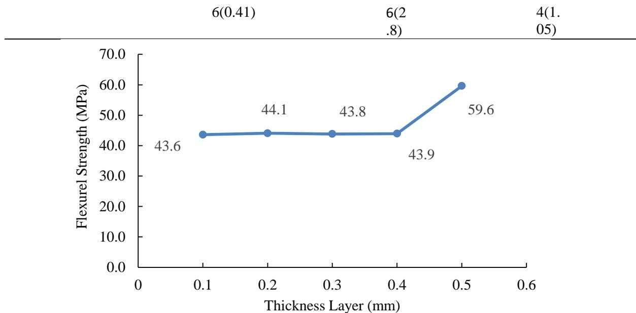
**Figure 7.** Graphical comparison of average maximum flexural strength ( $\sigma_f$ ) for the flexurel specimens as a function of layer thickness.
