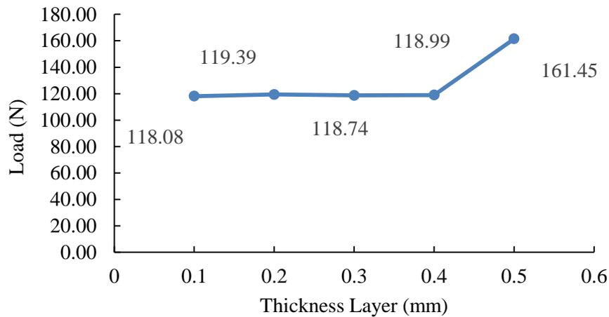
**Figure 9.** Graphical comparison of average maximum Load ( $P$ ) for the flexural specimens as a function of layer thickness.
