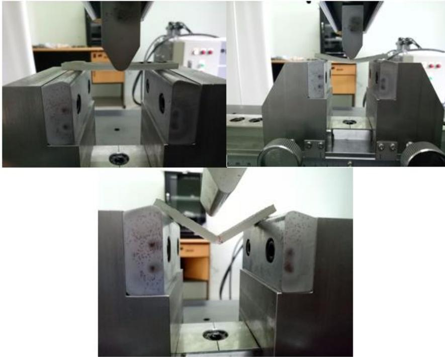
**Figure 6.** Three-point bending test.
