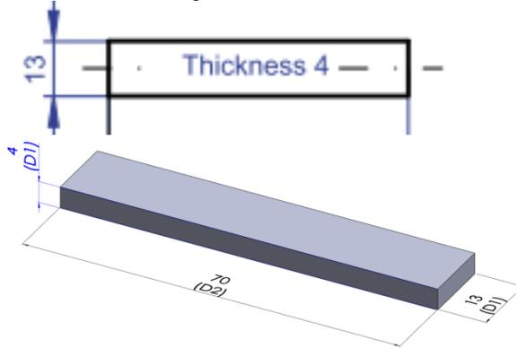
**Figure 4.** Standard specimens for 3-point bending specimen and dimensions are in mm [16].
