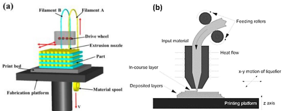
**Figure 1.** Schematic representation of typical [1]: (a) FDM setup (b) a Fused Filament Fabrication process.
