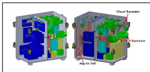
Fig. 3.1. Equipment arrangement inside of the satellite
