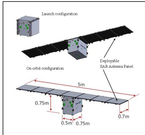
Fig. 2.1. Overview of small satellite with X-band SAR
