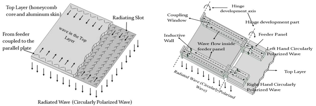
Fig.2.2. (a) Antenna panel from feeder side.
