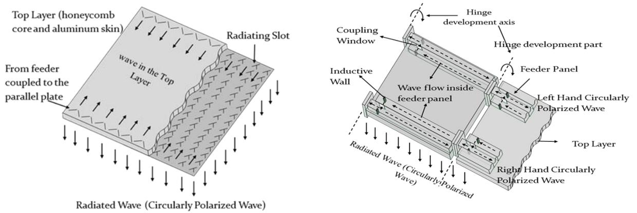
Fig.2.2. (a) Antenna panel from feeder side.
