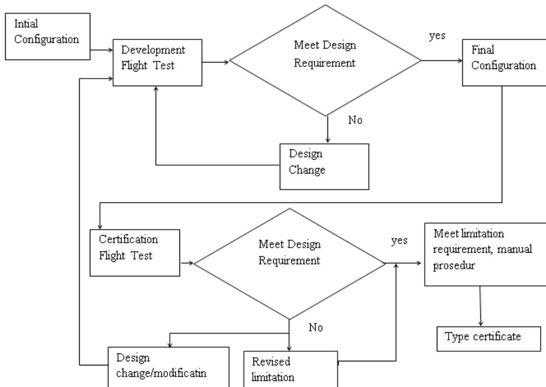
Fig. 2.1. Several step related to flight test activity to get type certificate
