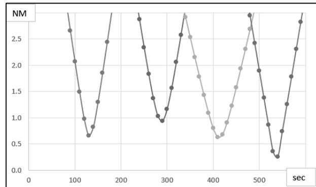
Fig. 5.1.2. Distance between UAV and intruder aircraft without maneuvers
