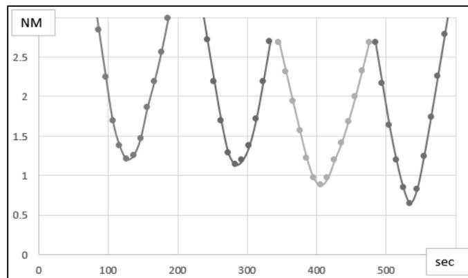
Fig. 5.1.4. Distance between UAV and intruder aircraft after avoidance maneuvers
