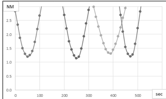
Fig. 5.2.4. Distance between UAV and intruder aircraft after avoidance maneuvers
