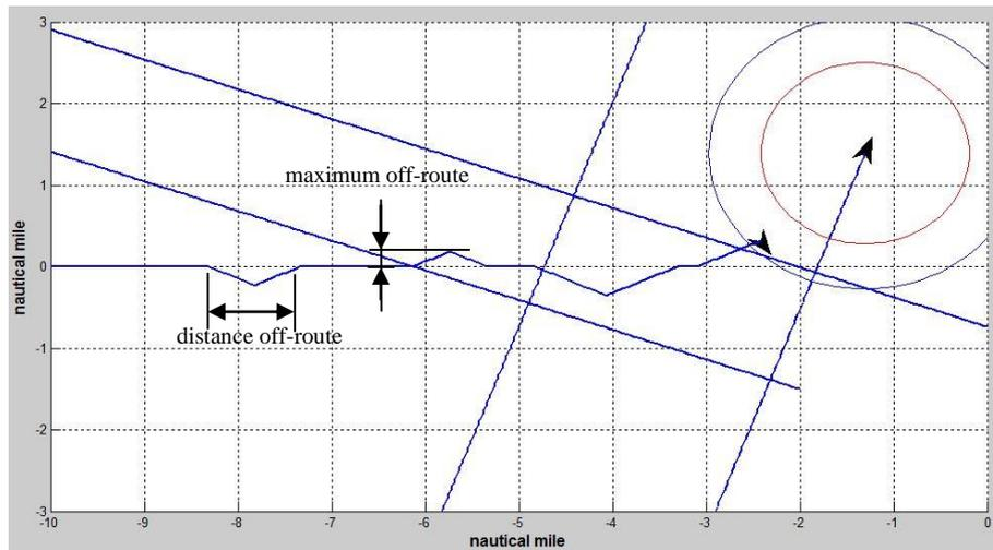
Fig. 5.1.3. Example screenshot of the UAV flight trajectory avoiding collision (first scenario)
