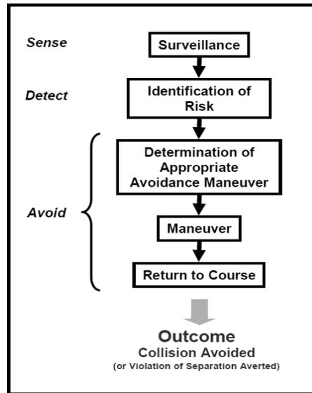
Fig. 2.1. Generic process model of collision avoidance algorithm<sup>3)</sup>
