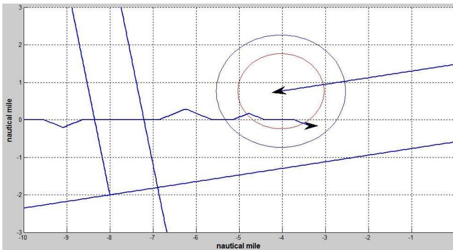
Fig. 5.2.3. Example screenshot of UAV flight trajectory avoiding collision (second scenario)
