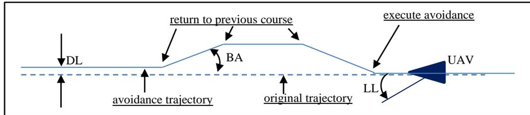
Fig. 4.1. Definitions for collision avoidance maneuver.
