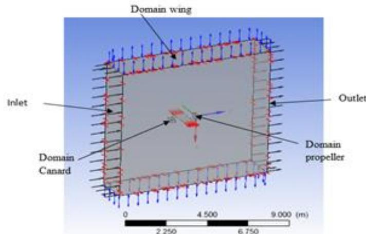
Fig. 3.3.2. Computational domain used in the simulation
