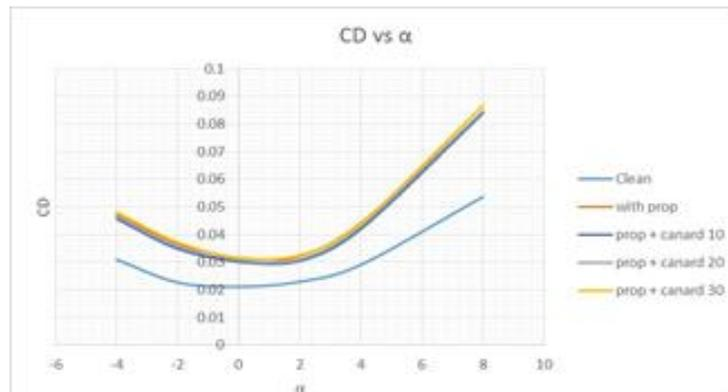
Fig. 4.3.2.1. Drag coefficient vs angle of attack comparison graph
