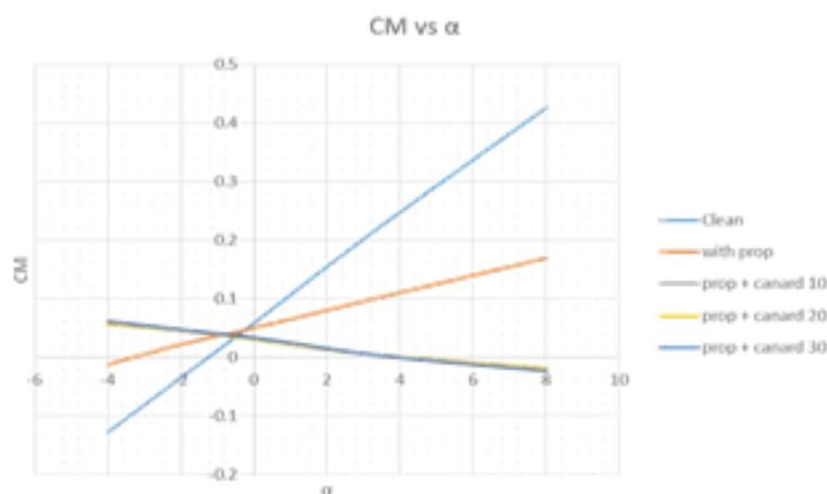
Fig. 4.3.3.1. Pitching moment coefficient vs angle of attack comparison graph
