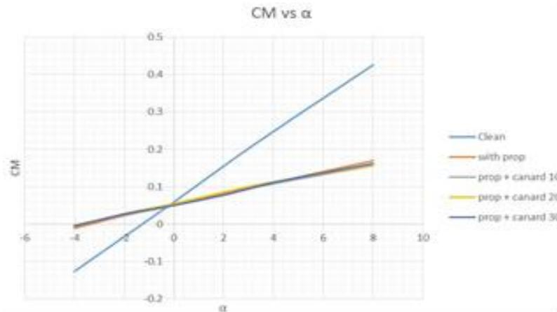
Fig. 4.1.3.1. Pitching moment coefficient vs angle of attack comparison graph
