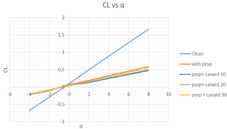
Fig. 4.1.1.1. Lift coefficient vs angle of attack comparison graph
