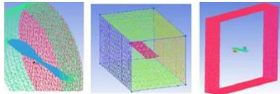
Fig. 3.3.1. Computational domains and generated meshes for propeller (left), canard (center), wing (right)
