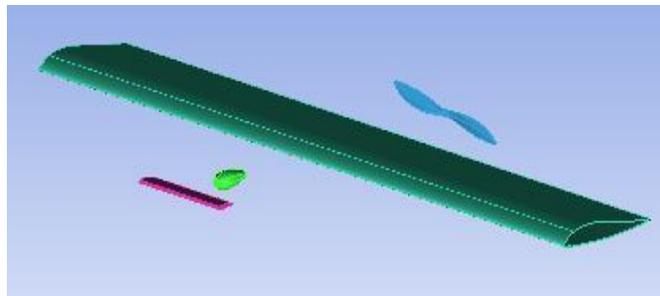
Fig. 4.2.2.3. Computational model of HALE UAV with new configuration
