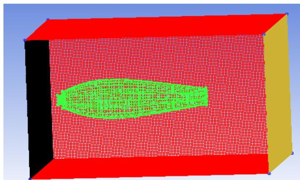
Fig. 4.2.2.1. Computational domain and mesh for the battery and its case
