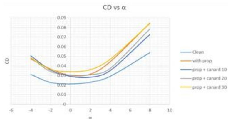
Fig. 4.1.2.1. Drag coefficient vs angle of attack comparison graph
