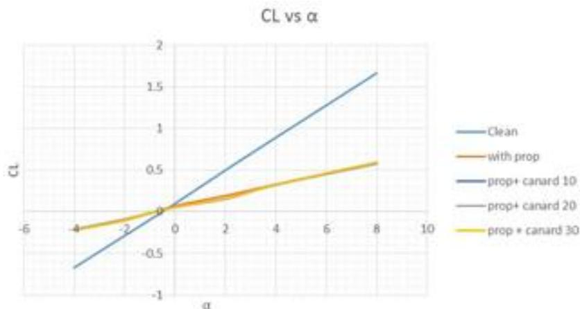
Fig. 4.3.1.1. Lift coefficient vs angle of attack comparison graph
