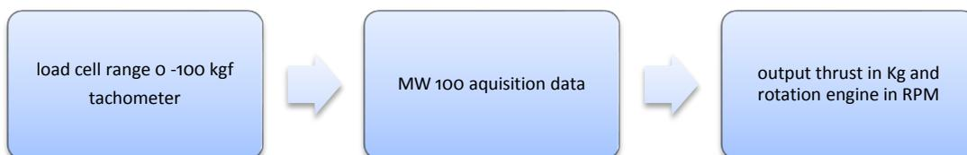
Figure 6 Illustration of measurement process of engine testing
