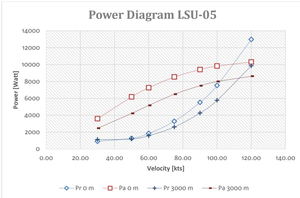
Figure 4 Power Required and Power Available Curve of LSU-05 using Propeller 28x10
