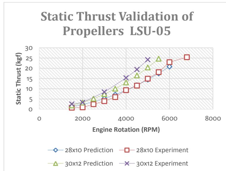
Figure 7. Result Data of Propeller Static Thrust Test; Propeller 28x10
