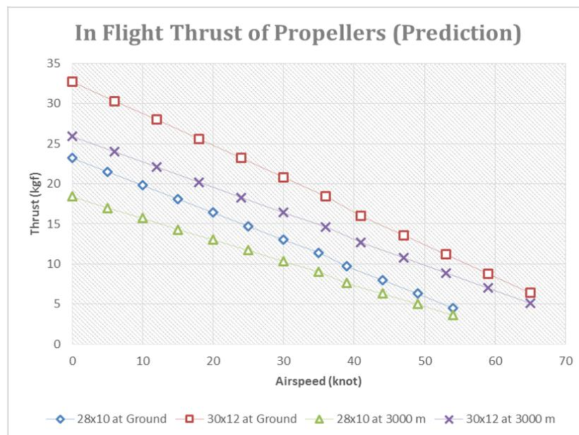
Figure 3 Thrust Curve of Propeller 28x10
