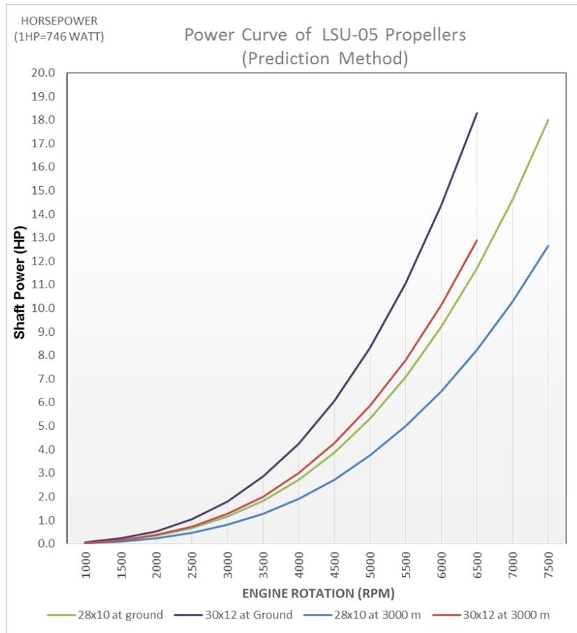
Figure 2. Shaft Power Curves of Propeller 28x10
