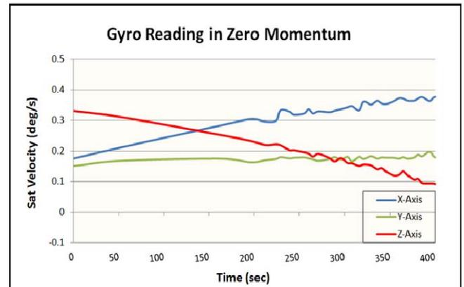
Fig. 3. Gyro Reading during Free Tumbling Condition
