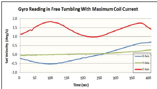
Fig. 5. Gyro Reading during Free Tumbling Condition with the Maximum Current Setting on Y Coil
