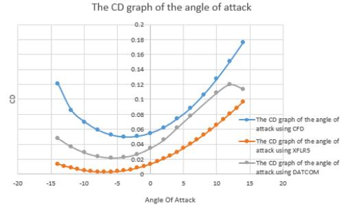
FIGURE 11. The  $C_D$  graph of angle of attack
