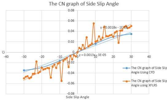
FIGURE 14. The  $C_n$  graph of the side slip angle
