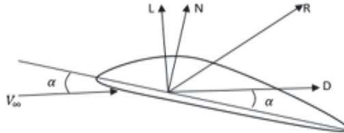
FIGURE 1. The resultant of force and its components
