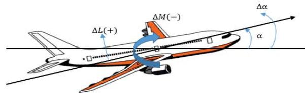
FIGURE 4. Longitudinal static stability illustration
