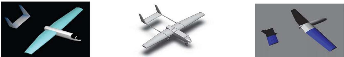
FIGURE 6. LSU 05-NG model with XFLR5, CFD and DATCOM
