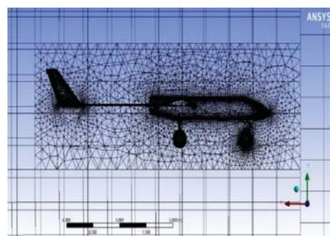
FIGURE 8. Meshing results with CFX ANSYS
