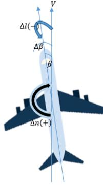
**FIGURE 5.** Lateral-directional static stability illustration
