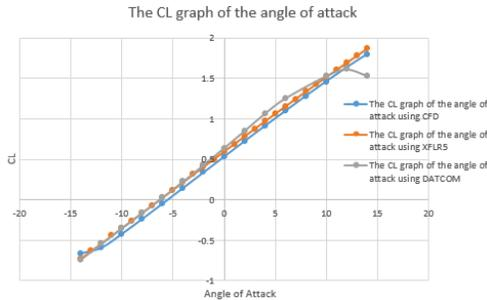
FIGURE 10. The  $C_L$  graph of the angle of attack
