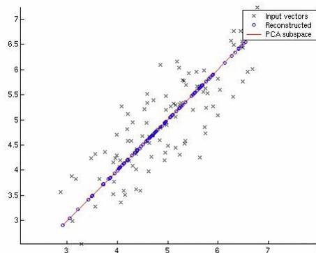
Figure 2-1. Principal Component Analysis used to find the best input variable with the minimal reconstruction error.
