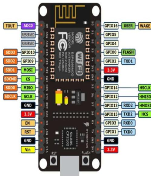
Figure 2. Layout module nodeMCU ESP8266
