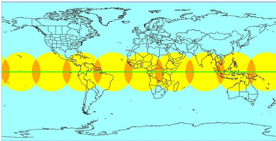
**Figure 1.** Concept of equatorial low earth satellite communication constellation.
