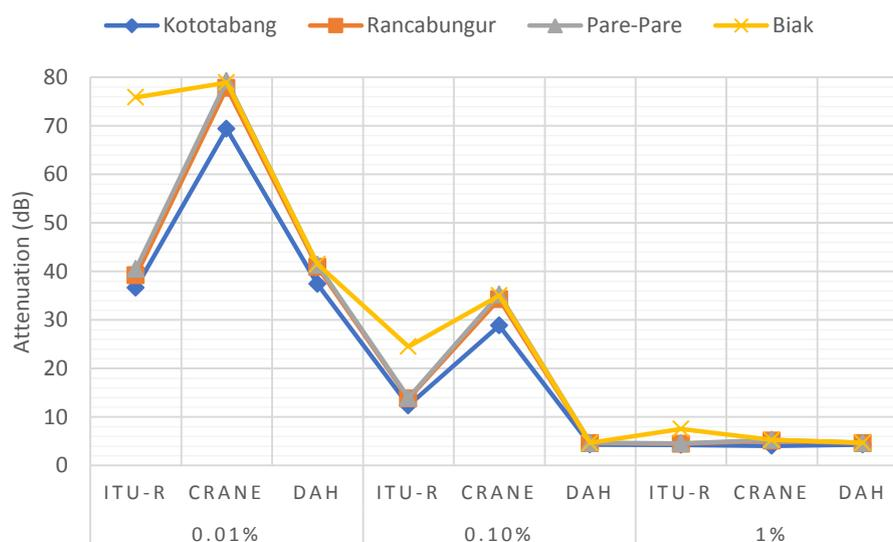
**Figure 2.** Variation of attenuation value using ITU-R, Crane, and DAH.
