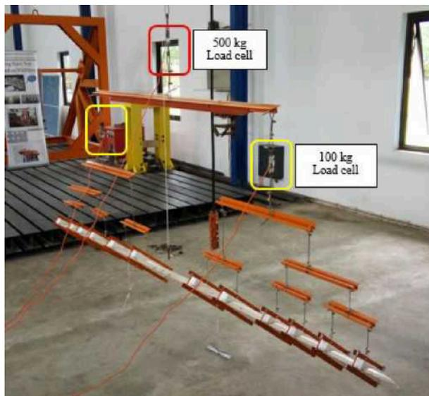
**FIGURE 5.** Load cell location on whiffletree
