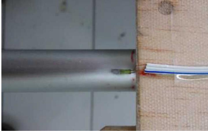
**FIGURE 4.** Strain gauge mounted on aluminum spar
