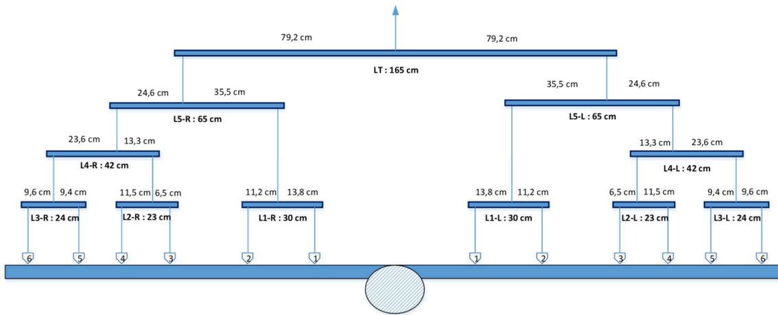
**FIGURE 2.** Whiffletree design for wing static test
