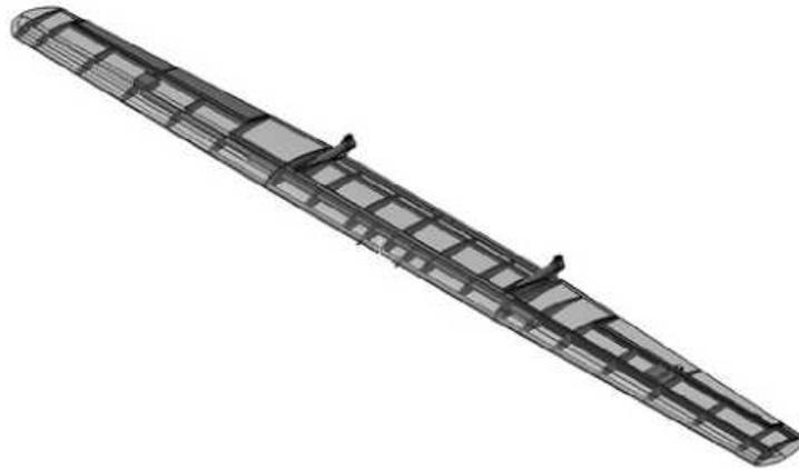
**FIGURE 1.** Design structure of LSU-02 NG LD wing
