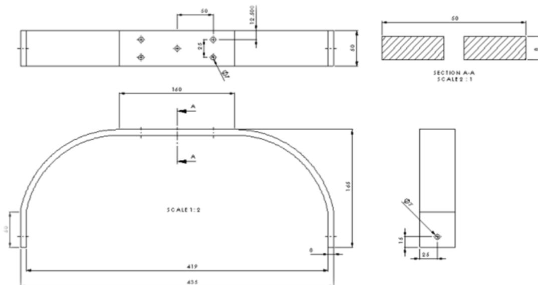
Fig. 5. Main Landing Gear Structure Dimension of LSU-02-02
