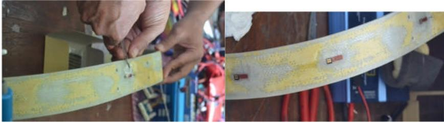
Fig. 6. Strain gauge placement process on MLG
