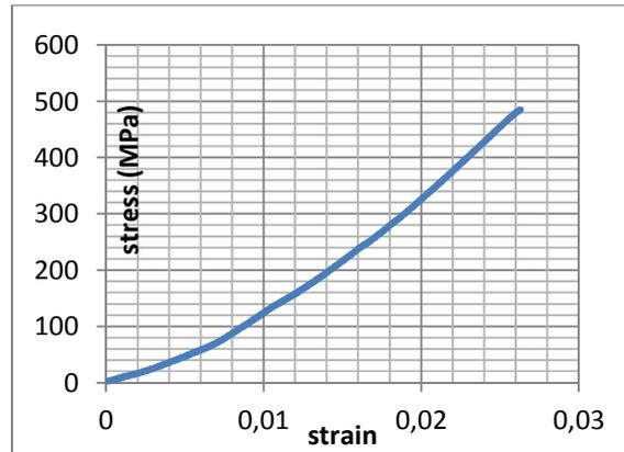
Fig. 1. Relationship stress - strain on tensile testing of e-glass composite UD 0<sup>0</sup>
