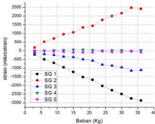
Fig. 12. Comparison of load and strain
