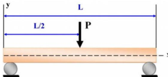
Fig. 2. Three point bending test
