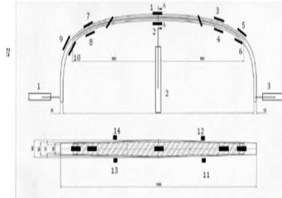
Fig. 4. Vertical static testing scheme's Main Landing Gear at BPPT<sup>8)</sup>
