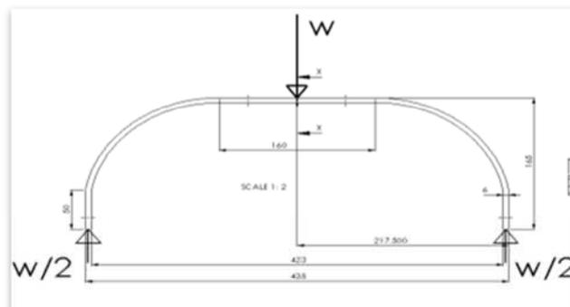
Fig. 8. Loads on the main landing gear LSU-02-02
