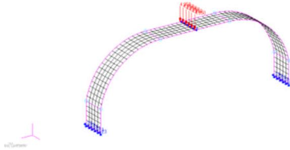
Fig. 9. Meshing and boundary conditions simulated loading
