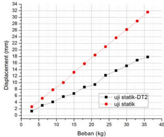
Fig. 15. Comparison of load and displacement
