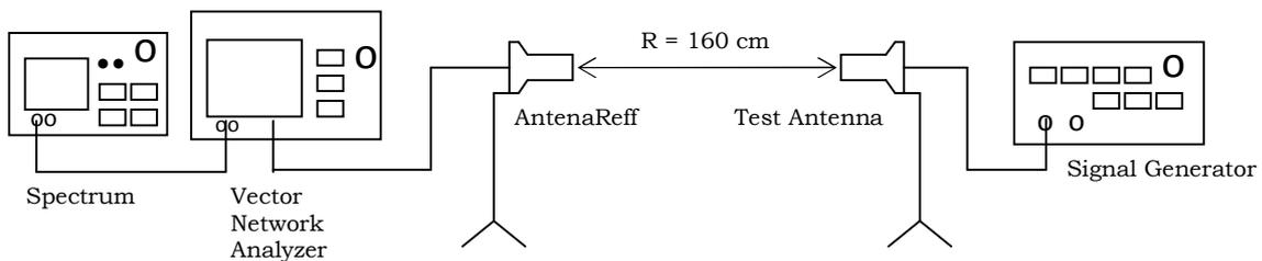
Fig. 7. Gain Test Procedure
