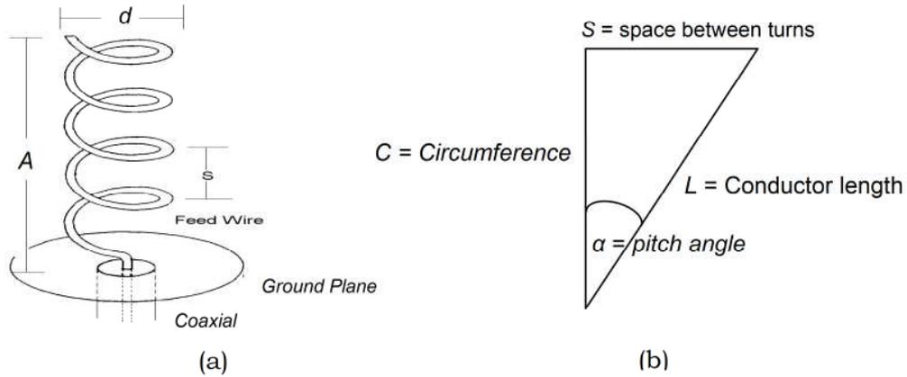
Fig. 1. (a) Helix antenna geometry, (b) Relation between circumference (C), diameter (d), pitch angle ( $\alpha$ ), space between turns (S) and the Helix length between loop (L)
