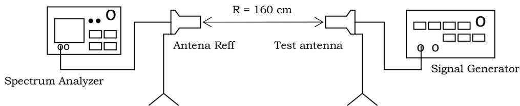
Fig. 6. Beamwidth Test Procedure
