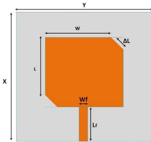
Fig. 3. Truncated Corner Microstrip Antenna Design
