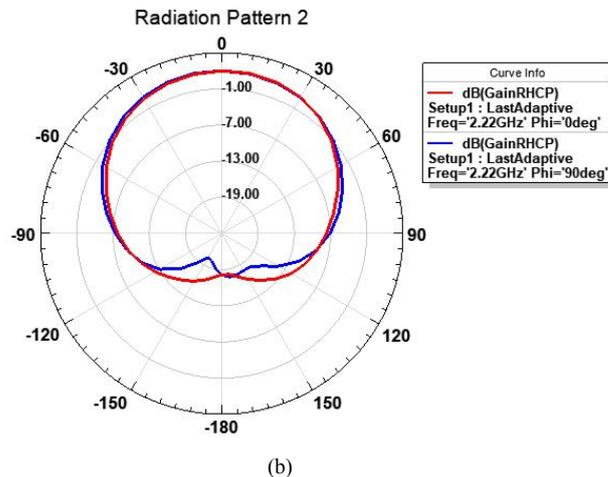
Fig. 9. (a) LHCP and (b) RHCP Gain of Antena Truncated Corner
