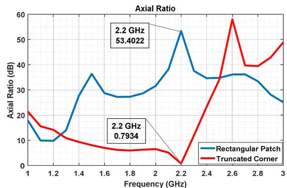
Fig. 7. Axial Ratio of Rectangular Patch & Truncated Corner
