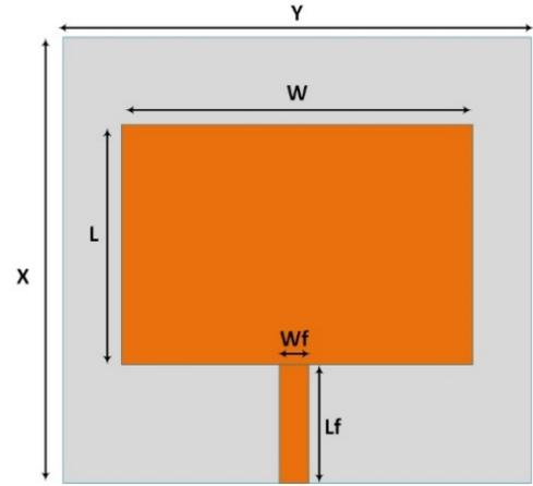
Fig. 2. Rectangular Patch Microstrip Antenna Design
