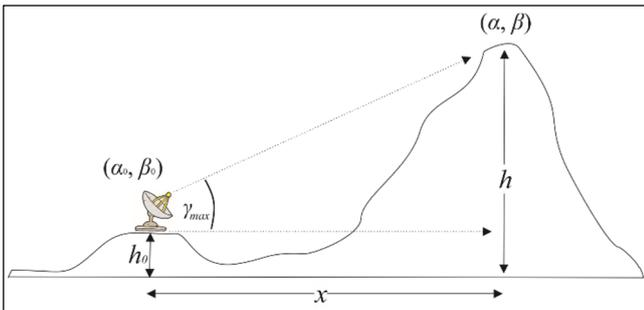
Fig. 2. Illustration of elevation blockage calculation.
