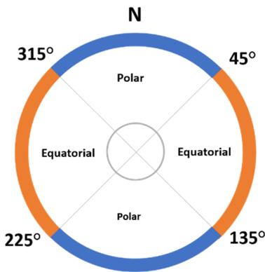
Fig. 6. Illustration of azimuth range for equatorial and polar-orbiting satellites.
