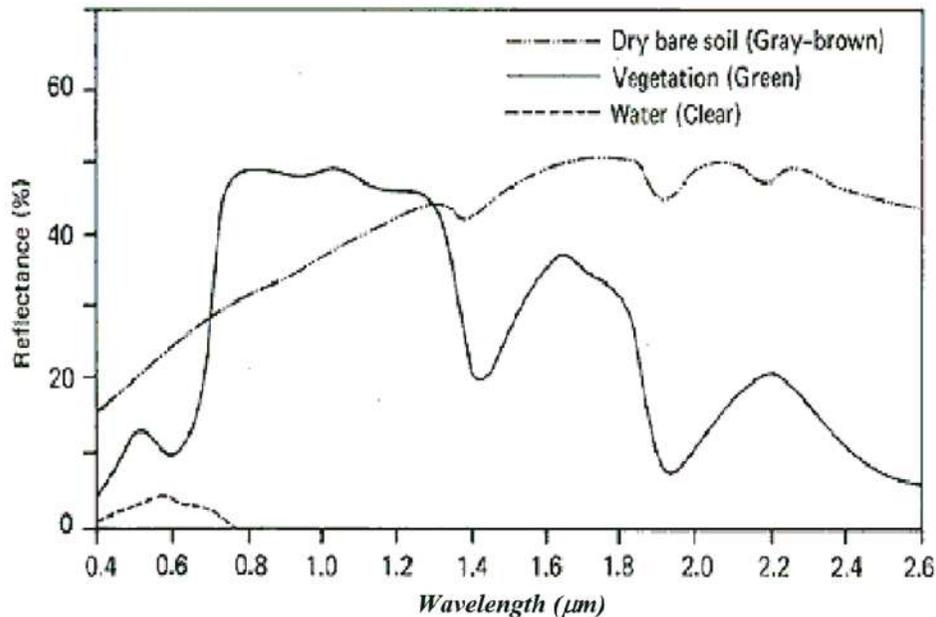
**Figure 3.** General Spectral Response of Water, Bare Soil, and Vegetation object
