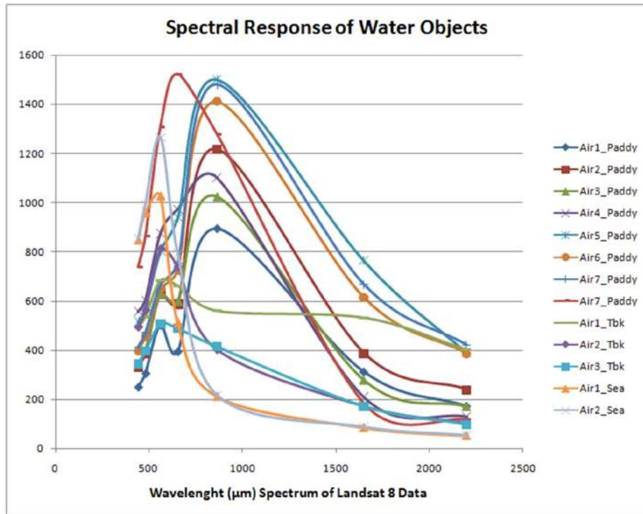
**Figure 11.** Spectral Response of Water Object in Paddy Field, Fishpond, and Sea Based on Landsat 8 Data
