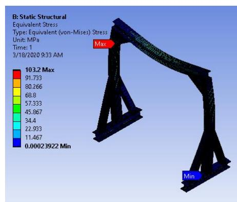
Figure 5. The von Mises stress of gantry crane structure with a load capacity of 7 tons
