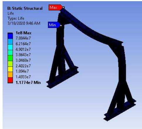
Figure 8. The fatigue life prediction of the gantry crane structure with a load capacity of 7 tons.
