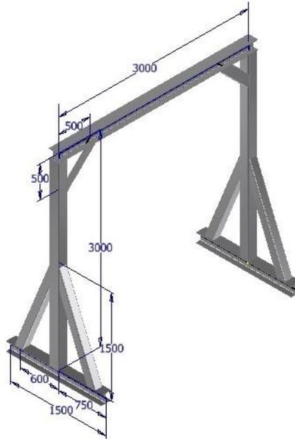
**Figure 2.** Structure dimensions of gantry crane capacity of 9 tons (in mm) [7].
