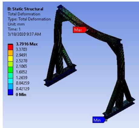
Figure 6. The deformation of gantry crane structure with a load capacity of 7 tons
