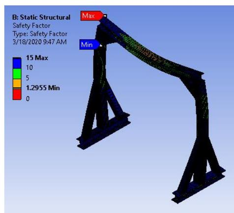
Figure 9. The safety factor of fatigue life of the gantry crane structure with a load capacity of 7 tons.
