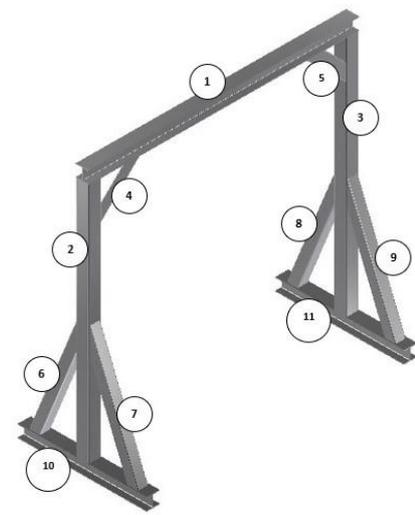
**Figure 1.** The 3D design of a 9-tons gantry crane structure [7].
