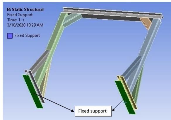
Figure 3. Fixed support location of the gantry crane structure.
