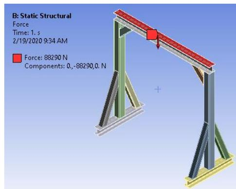
Figure 4. Location of loading of the gantry crane structure.
