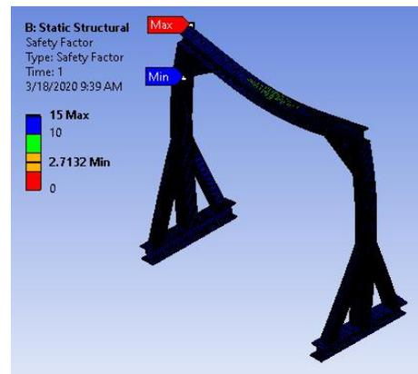
Figure 7. The safety factor of gantry crane structure with a load capacity of 7 tons.
